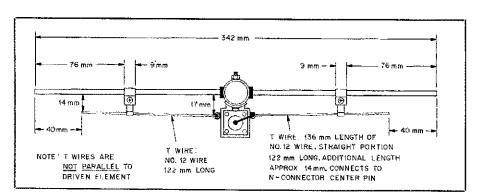
Fig 14—Details of the driven element and T match for the 33-element Yagi. See Fig 8 for additional information. Lengths are given in millimeters to allow precise duplication of the antenna. See text.
