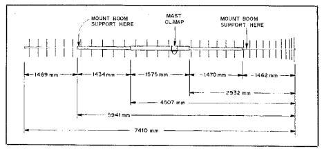
Fig 12—Boom-construction information for the K1FO 33-element Yagi. Lengths are given in millimeters to allow precise duplication of the antenna. See text.
