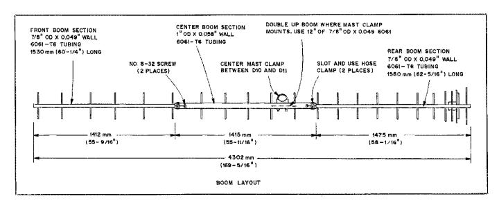
Fig 6—Boom-construction information for the K1FO 22-element Yagi. Lengths are given in millimeters to allow precise duplication of the antenna. See text.
