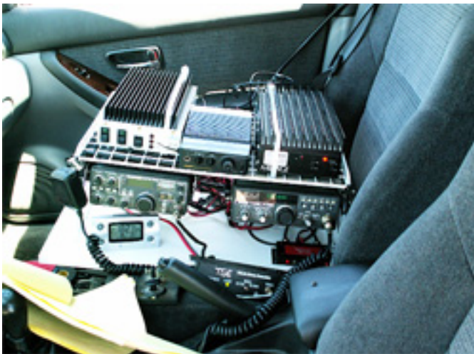
Photo 2 - Inside the rover, a Yaesu FT-780R drives a Mirage amp to 50 watts and a Kenwood TR-9130 and TE Systems amp provide 2 m liaison.
