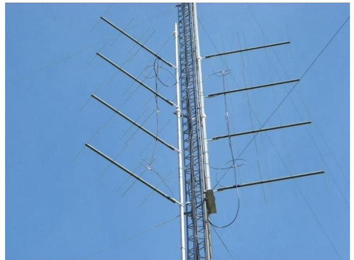
This pair of YU7EF 5-element rotatable Yagi stacks are located in Pennsylvania for remote operating by Stan, KA1ZE/3 from his Clearwater Beach, Florida home. (Photo by KA1ZE)
