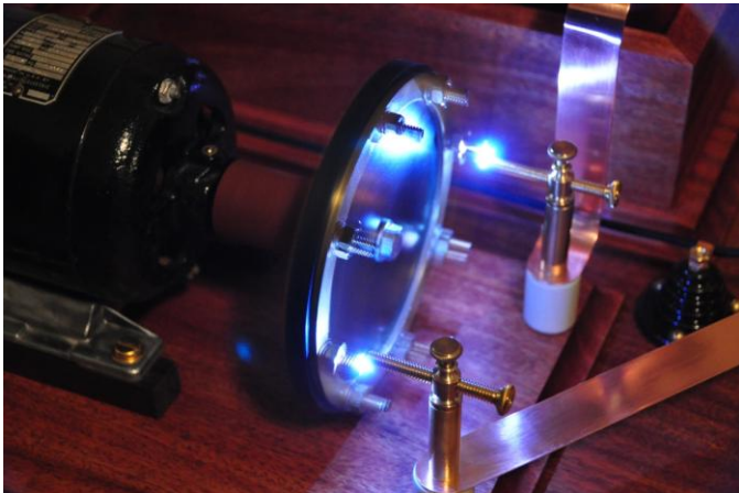
Figure 5. N4GG’s synchronous rotary gap firing at 2,000 amps
