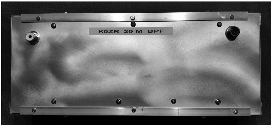
Figure 14 — The completed 20 m band pass filter. [Jeff Crawford, KØZR, photo]
