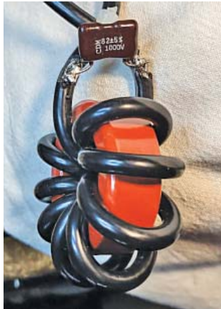
▲ Figure 3 — The tinned and tie-wrapped cable.
