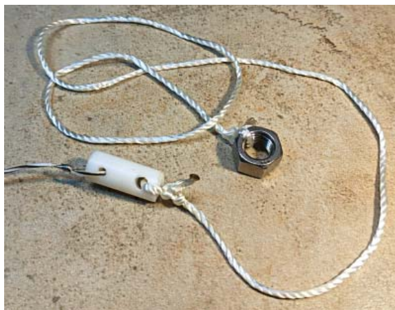
▲ Figure 6 — The wire and coax junction.
