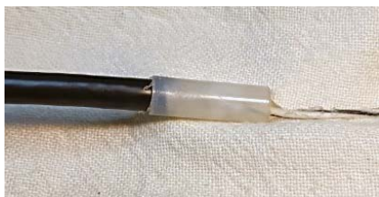
▲ Figure 6 — The wire and coax junction.
