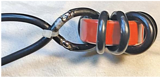
▲ Figure 3 — The tinned and tie-wrapped cable.
