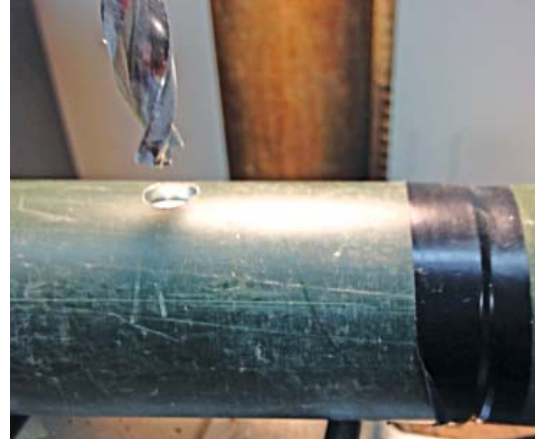
Figure 3 — Drill the hole through the female end of the mast by drilling through the existing hole in the male end.
