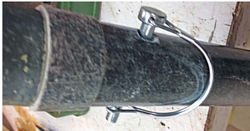
Figure 4 — The mast after holes are drilled and the hitch pins inserted.
