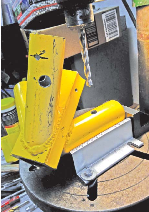
Figure 2 — Positioning a tripod leg for drilling.
