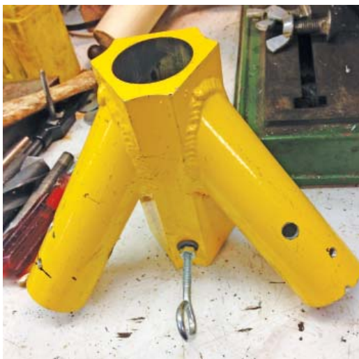
Figure 5 — Threaded eye bolt is screwed into a threaded hole in the vertical leg of the tripod.
