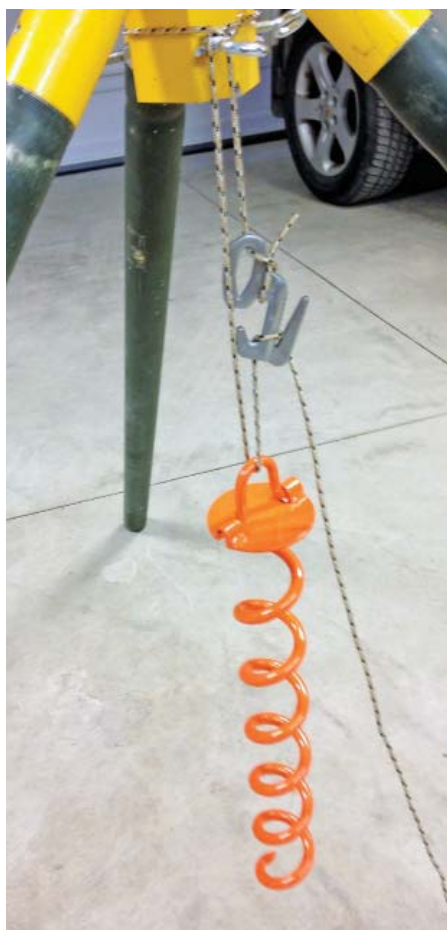
Figure 6 — A view of how the tripod rope tightener and ground anchor are connected together using paracord.
