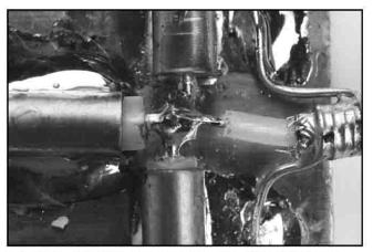
A close up of the T-junction connected to 50- $\Omega$  Teflon coax.
