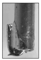
Here you can see how the center conductor is grounded to the shield.
