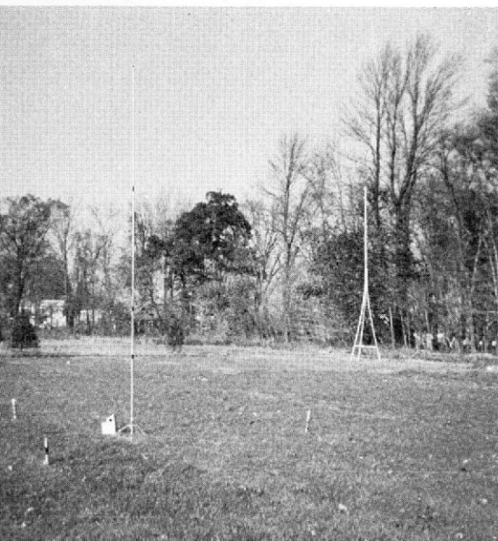
The 20-meter vertical antenna in the foreground, and the 26-foot test tower.
